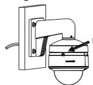
D: Fastening screw of dome camera
